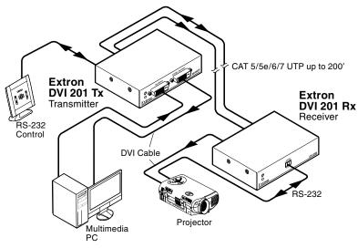
Figure 1-1 — Typical transmitter and receiver application
